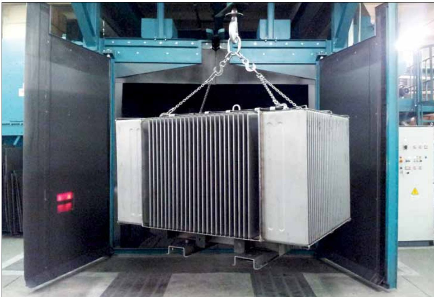
A Capri shot blasting machine at work with a bulky, densely finned tank
