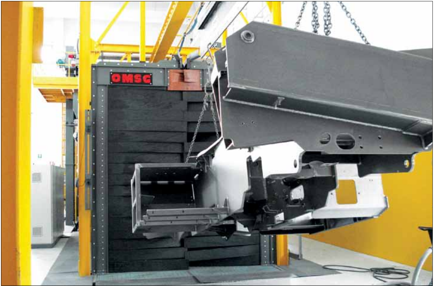
The complex chassis of a mobile crane
