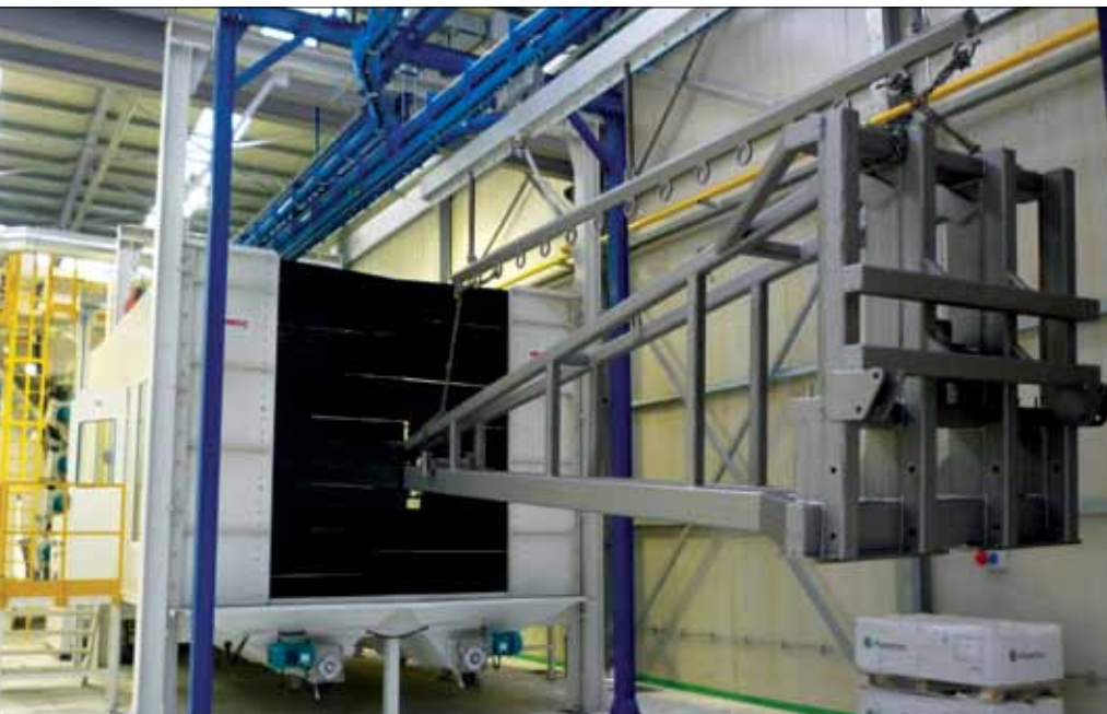
The structural arm of an agricultural machine at shot blasting exit
