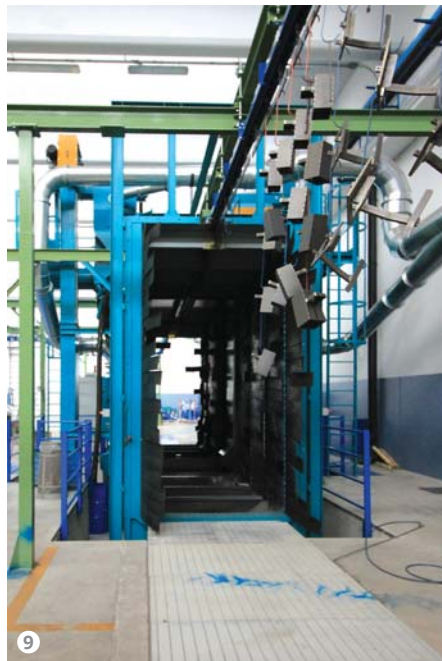
Figure 9: The abrasive can be recovered and reconditioned: through a blowing nozzle, the media left on the component are removed by the operator and collected in hoppers placed in the exit area.
