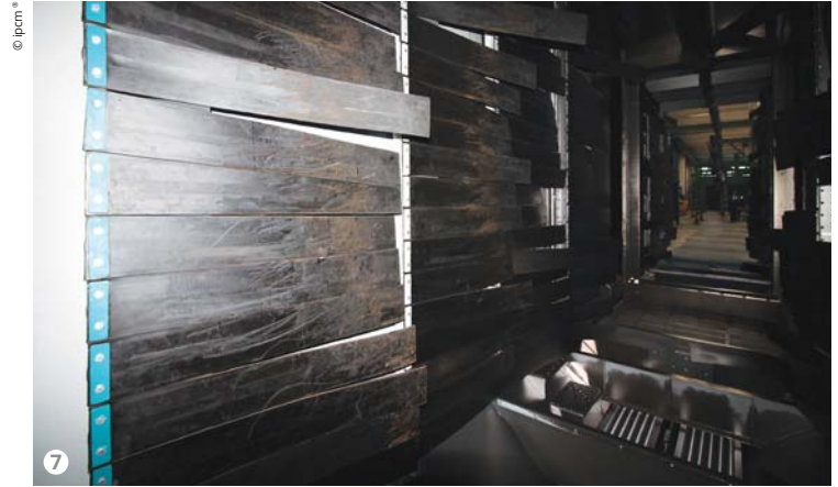
Figures 7 and 8: In order to perform a continuous flow process, the tunnel shot blasting system has no closing doors, but it is equipped with vestibules featuring rubber curtains at both the entrance and exit: this reduces the spillage of media and dust from the shot blasting chamber.
