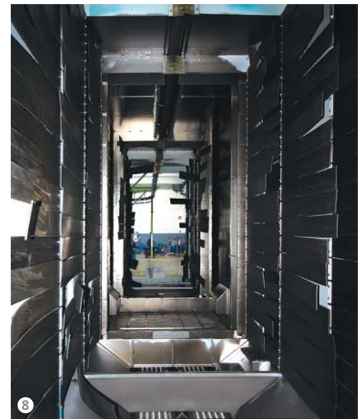
Figures 7 and 8: In order to perform a continuous flow process, the tunnel shot blasting system has no closing doors, but it is equipped with vestibules featuring rubber curtains at both the entrance and exit: this reduces the spillage of media and dust from the shot blasting chamber.
