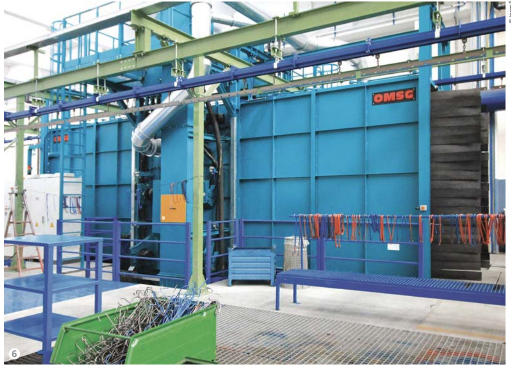
Figure 6: The TUNNELBLAST 1525/12 tunnel shot blasting system installed in December 2017 by OMSG (Villa Cortese, Milan).
