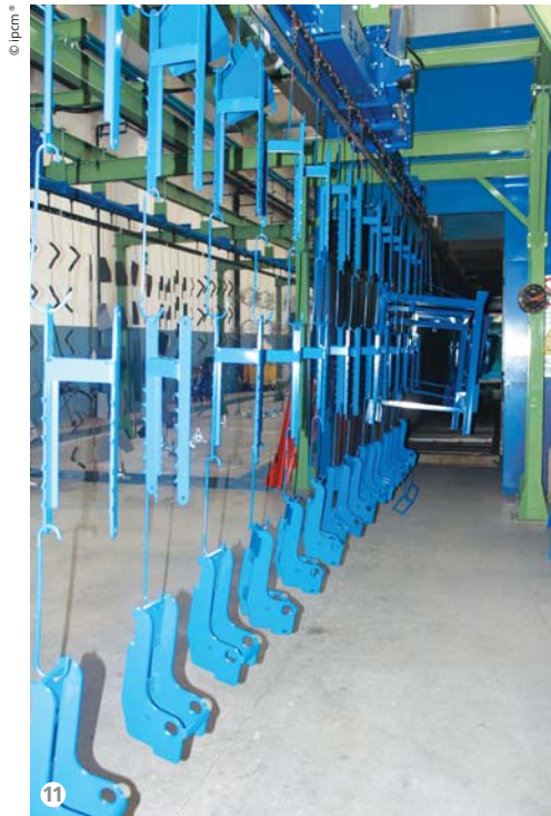
Figure 11: Workpieces entering the polymerisation oven.
