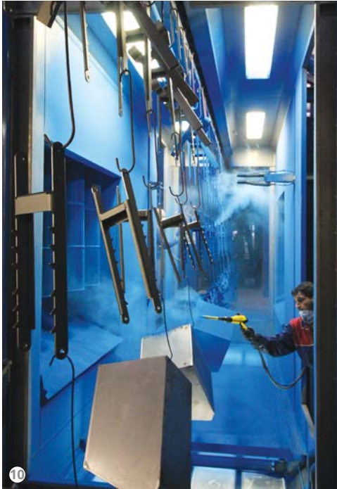
Figure 10: The powder coating booth is equipped with 4 reciprocators and 2 guns for manual retouching, supplied by Wagner; it applies Sherwin-Williams polyester powders.
