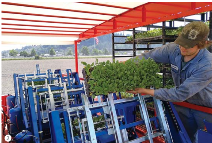
Figure 2: An automatic transplanting machine developed for vegetable plants placed in seed boxes.
