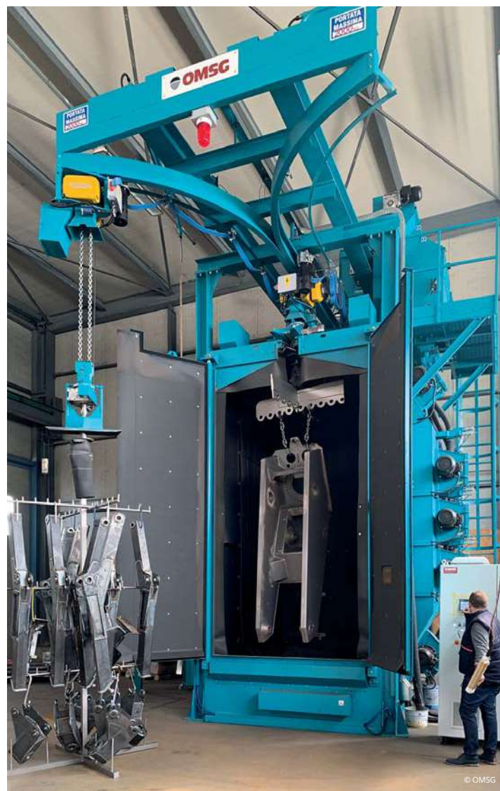
A component entering the new shot blasting system.
