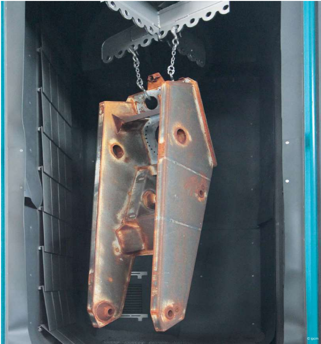
A detail of the sandblasting chamber.
