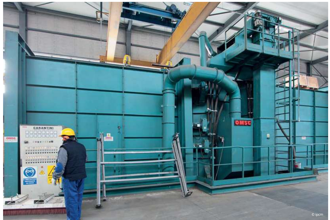
The Tunnelblast 2530/16 tunnel shot blasting plant installed by OMSG.
