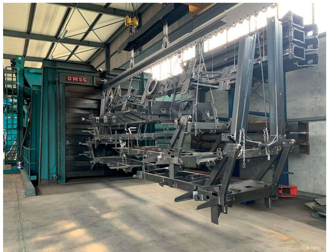
Some complex-shaped parts shot blasted by Carantini.
