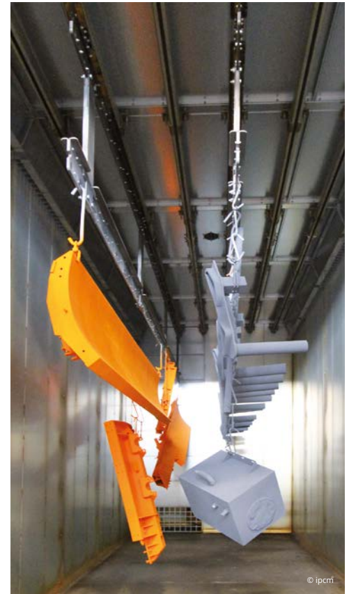
Coated parts inside one of the ovens.
