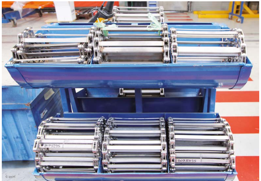
The metallic belt extraction system borrowed by Giletta from the agricultural machinery field is the key factor that determined the company’s success in this sector.
