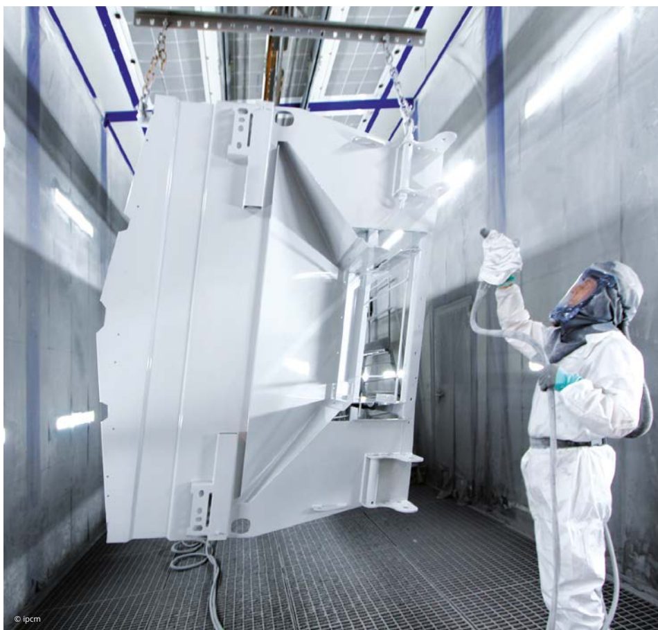
Liquid base coat application in one of the two vertical-flow pressurised booths.
